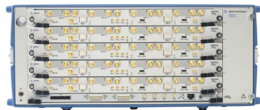
Figure 3. Five Agilent M9703A AXLe 12-bit digitizers installed in the Agilent M9505A 5-slot AXLe chassis to form a 40-channel 12-bit acquisition system.
